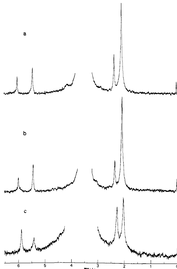
Figure 1. Pmr spectra of sodium acetylacetonate in pyridine- d 5 containing 18-crown-6: a, -50^\circ , crown/enolate ratio 1.6; b, -44^\circ , crown/enolate ratio 1.6; c, -50^\circ , crown/enolate ratio 3.7.
